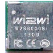
QFN Footprint: 6.75 mm x 6.75 mm x 2 mm
